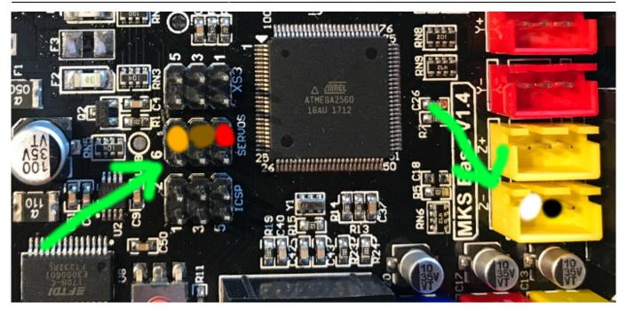
connect the BLTouch to the two sockets where the green arrows point to. Orange is S(ignal) pin, Brown is GND, Red is 5V, White is ZMIN and Black again GND. These are the lables you can see on the BLTouch sensor.
