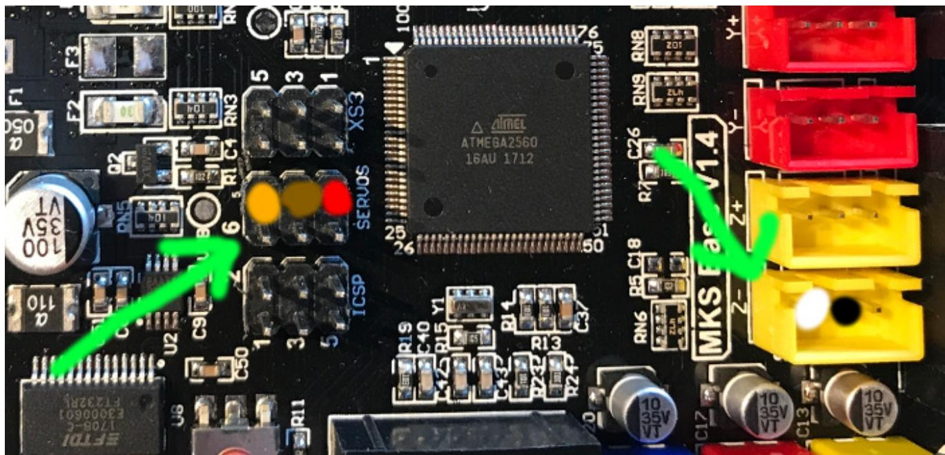
connect the BLTouch to the two sockets where the green arrows point to. Orange is S(signal) pin, Brown is GND, Red is 5V, White is ZMIN and Black again GND. These are the labels you can see on the BLTouch sensor.
