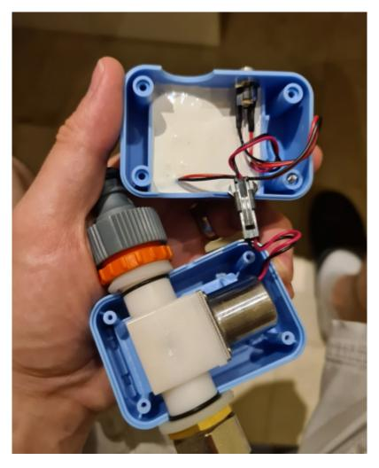
now remove the board by carefully cutting away some of the white silicone from the back and also remove the silicone where the pi header next to the button is
