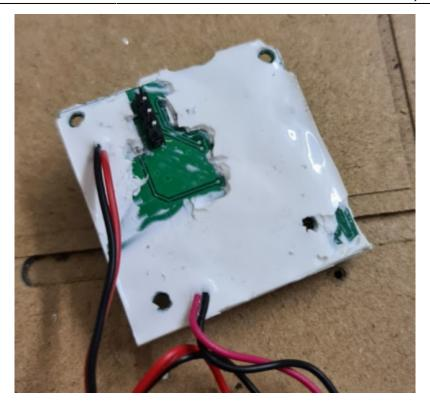
Pin header next to the button is used to re-program. the pinout is as follows (from pin closest to the outside edge of the board towards the inside of the board): 1.) GND 2.) TX 3.) RX 4.) 3.3V
