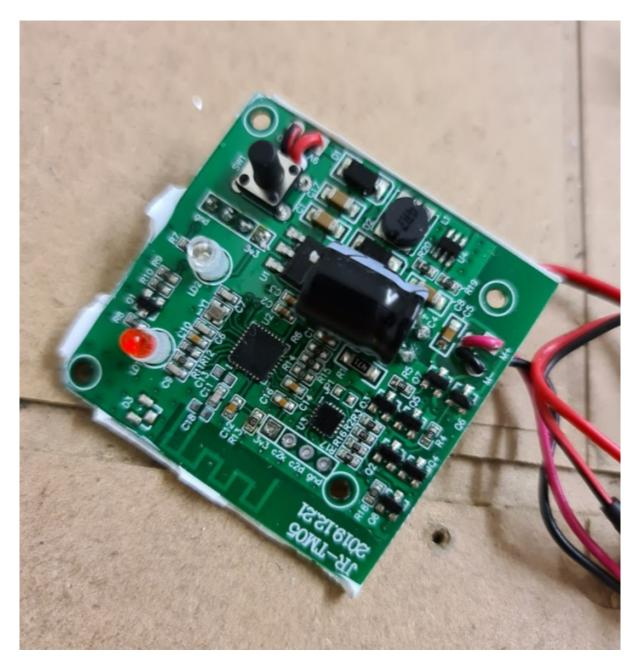
luckily the only button on the board is connected to GPIO0 which makes it also the flash-mode switch :)
